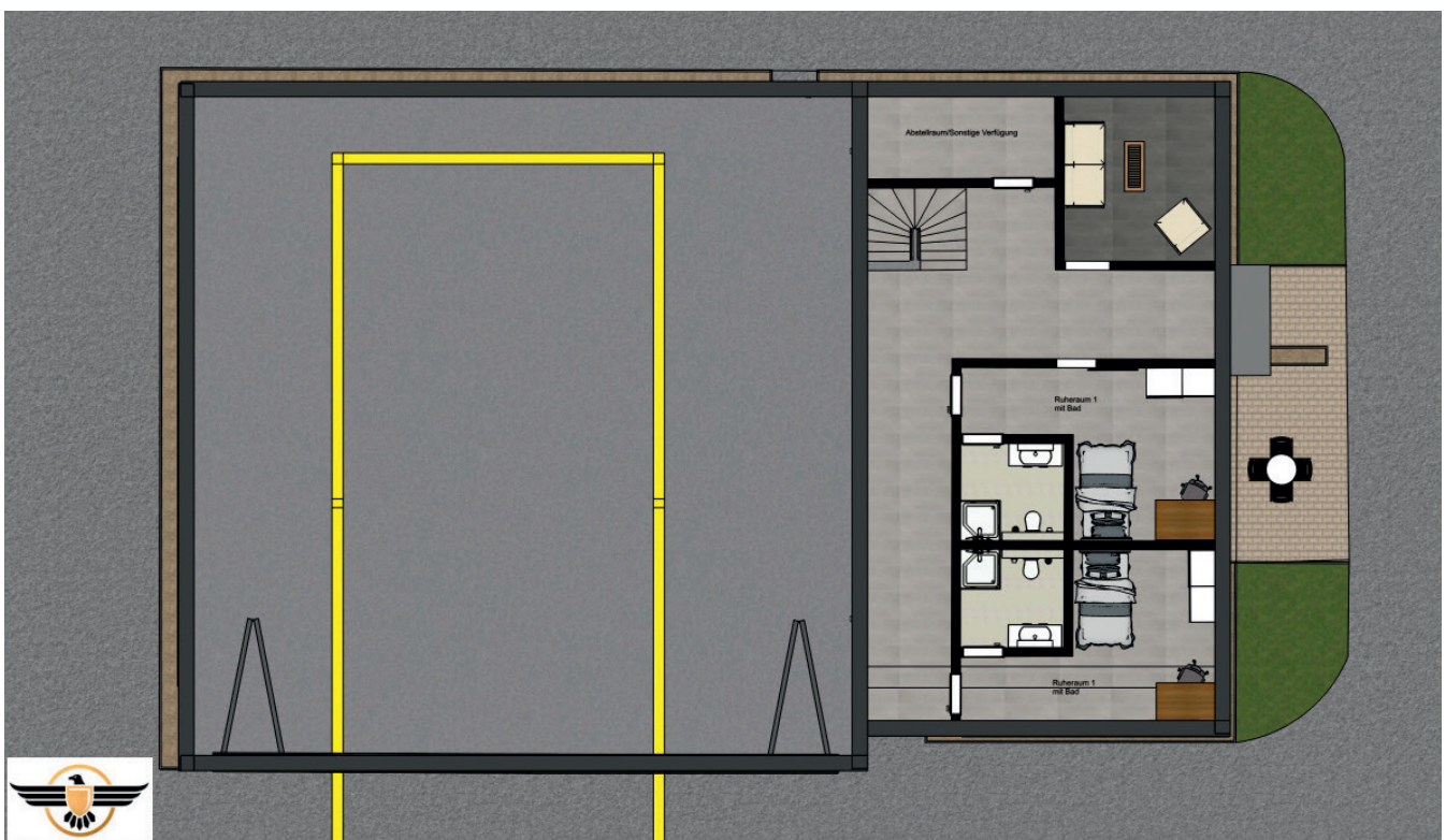
Figure 5.18: Example of a solid construction building as a long-term solution for a multicopter station (Floor plan upper floor)
