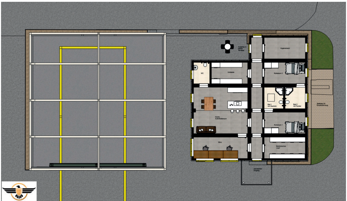
Figure 5.14: Example of a container station as a flexible solution for a multicopter station (Floor plan)
