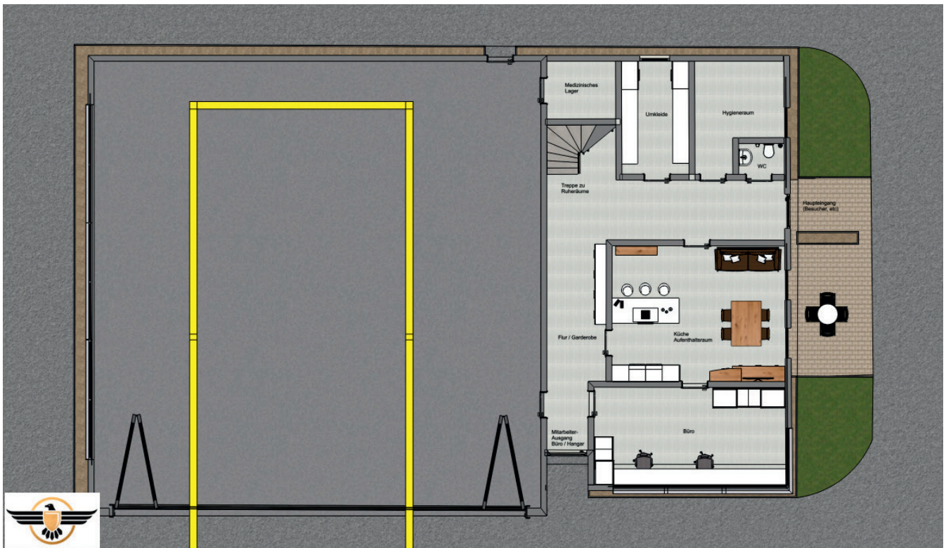
Figure 5.17: Example of a solid construction building as a long-term solution for a multicopter station (Ground floor plan)
